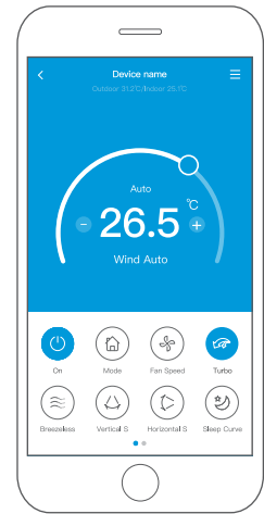
③ Thus, user can control air conditioners on/off status, operation mode, temperature, fan speed and so on.
